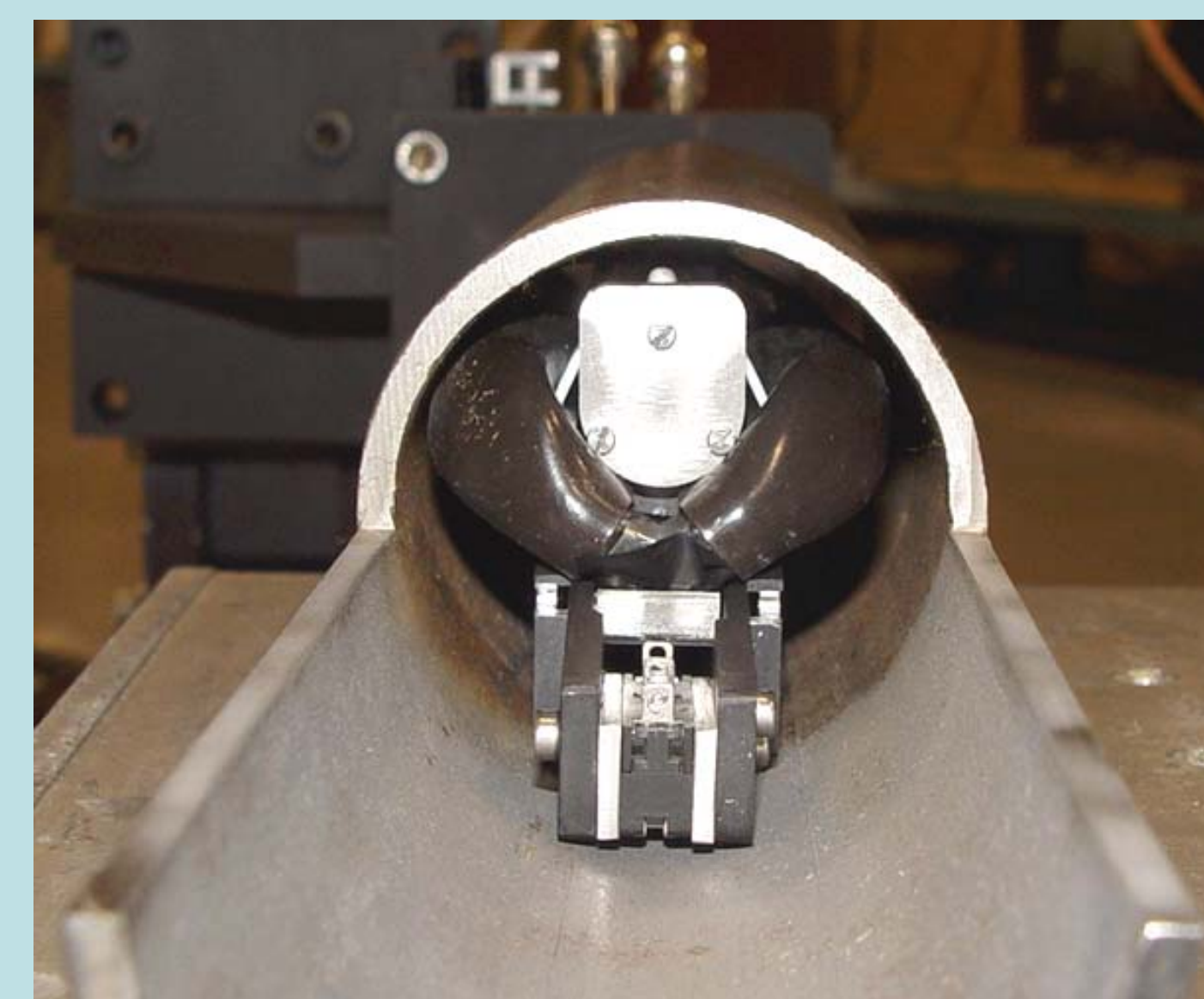
MG15P goniometer measuring residual stress inside a 50 mm bore.
