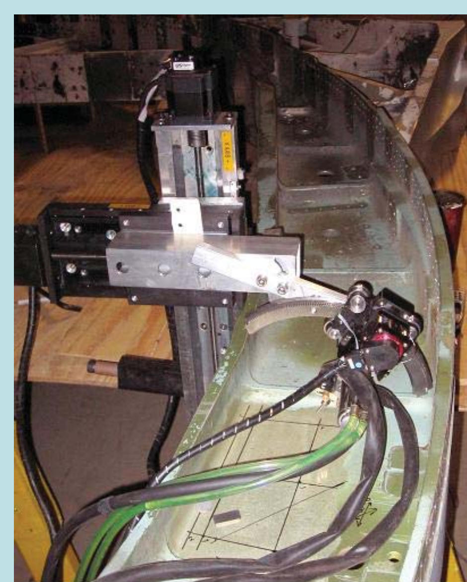
MGR40P goniometer measuring residual stress on an uninstalled aircraft frame.
