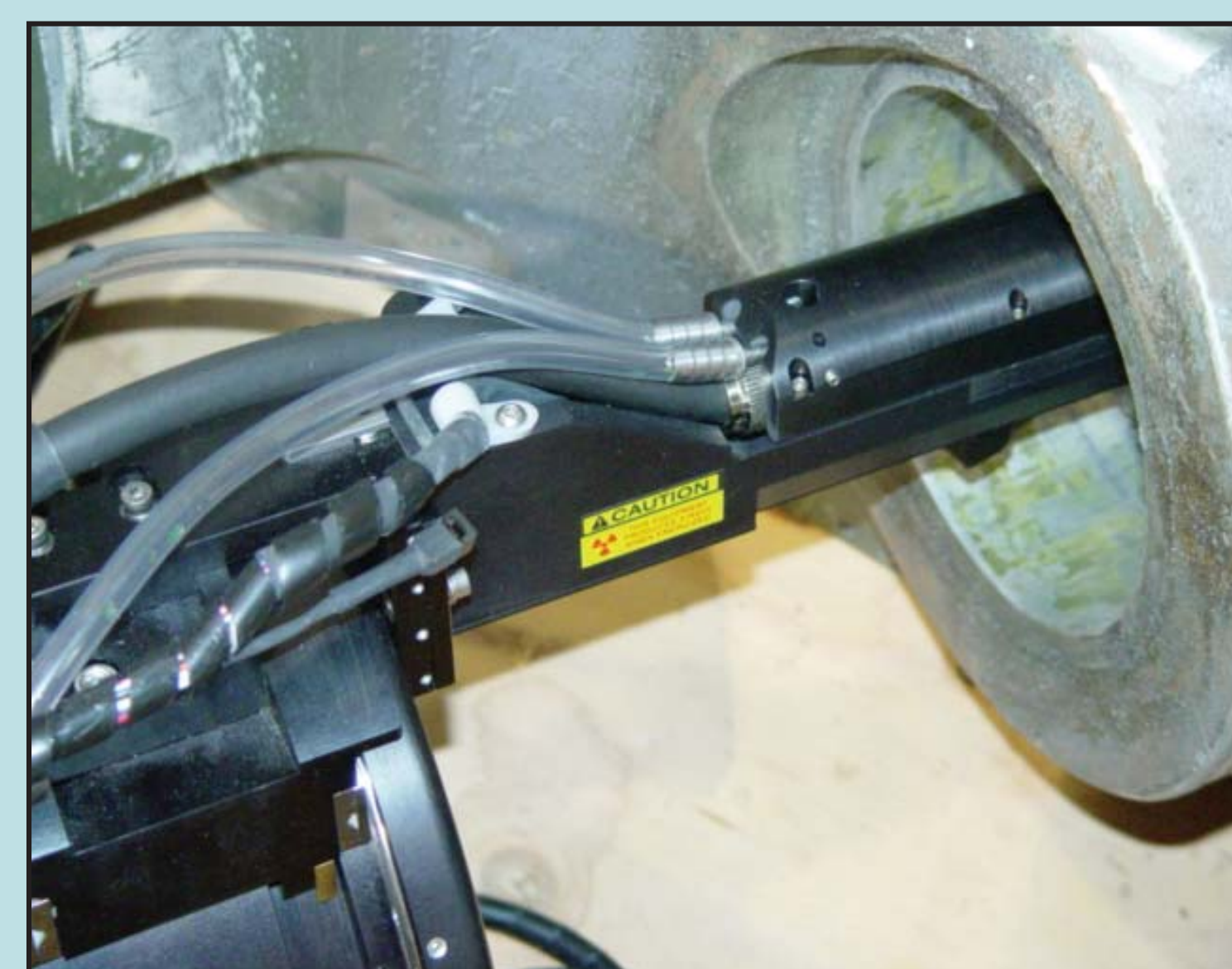
MG30P goniometer measuring residual hoop stresses inside a trunion.
